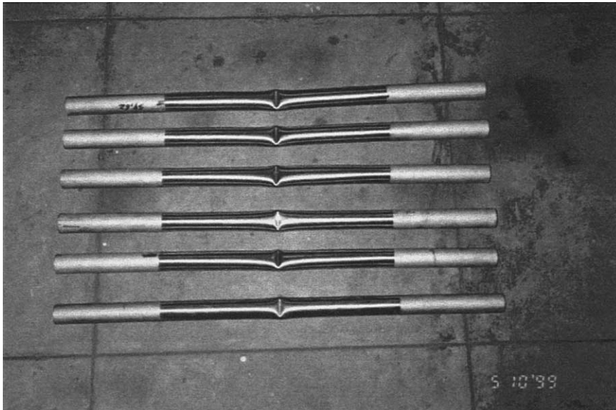
Fig. 10. A picture of the local buckling for some 304 stainless steel tubes.
